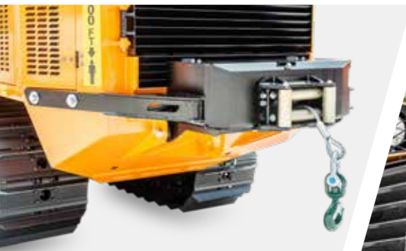
Rear winch - rated towing capacity: 6t
