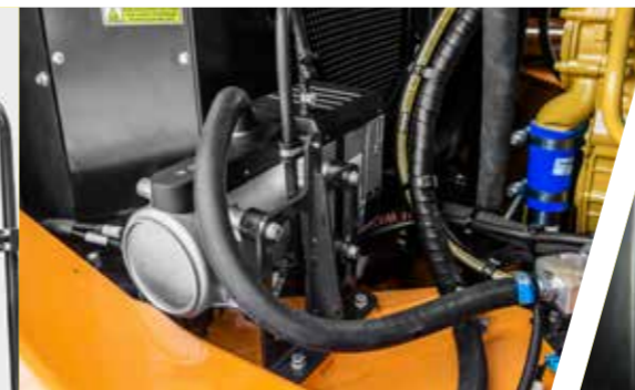
Pre-heating system for engine and hydraulic oil
