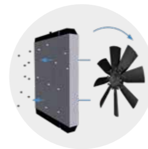
A reversible fan maximizes radiator efficiency (4)
