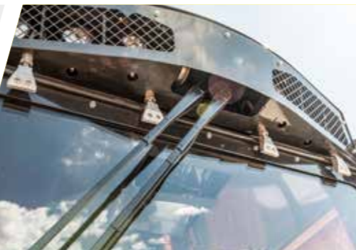
Air-window cleaning system
