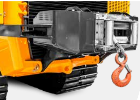
Rear winch - rated towing capacity: 6t
