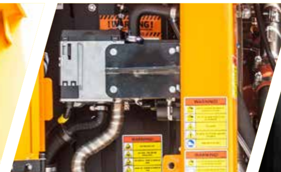
Pre-heating system for engine and hydraulic oil
