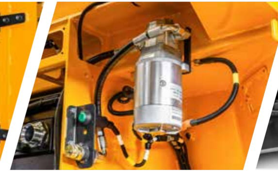
Oil top-off pump (service package)
