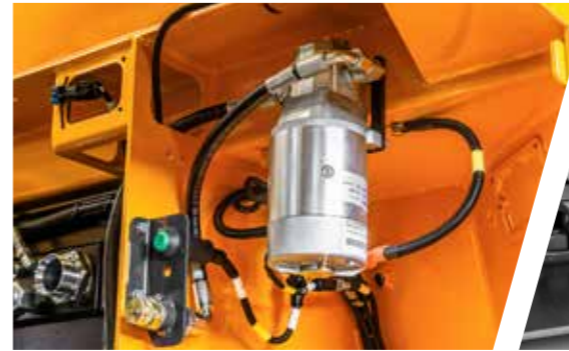
Oil top-off pump (service package)
