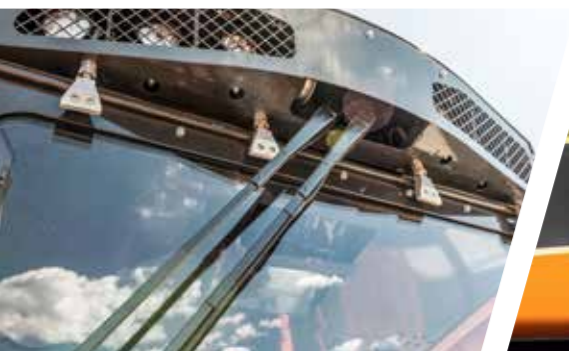
Air-window cleaning system
