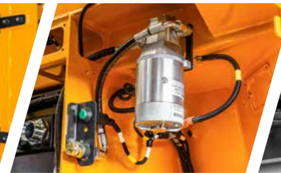
Oil top-off pump (service package)
