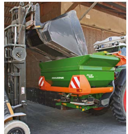
Filling with an industrial front loading shovel
