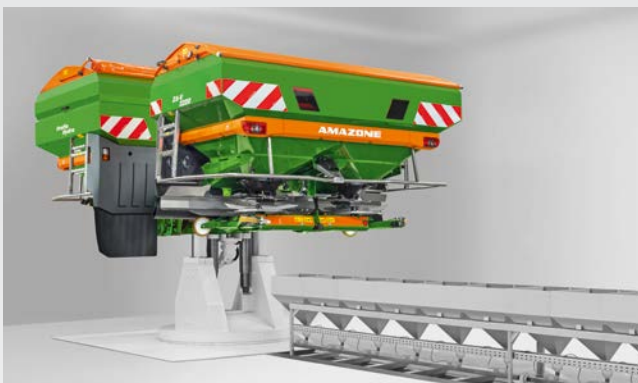
Modern fertiliser spreader test hall
