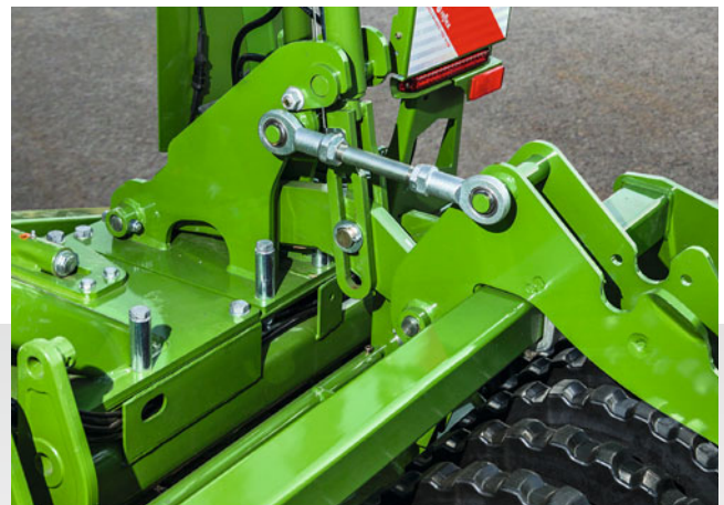
✔ Parallel guidance of the roller
