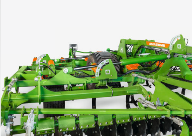
Working depth display for the three soil-engaging elements
