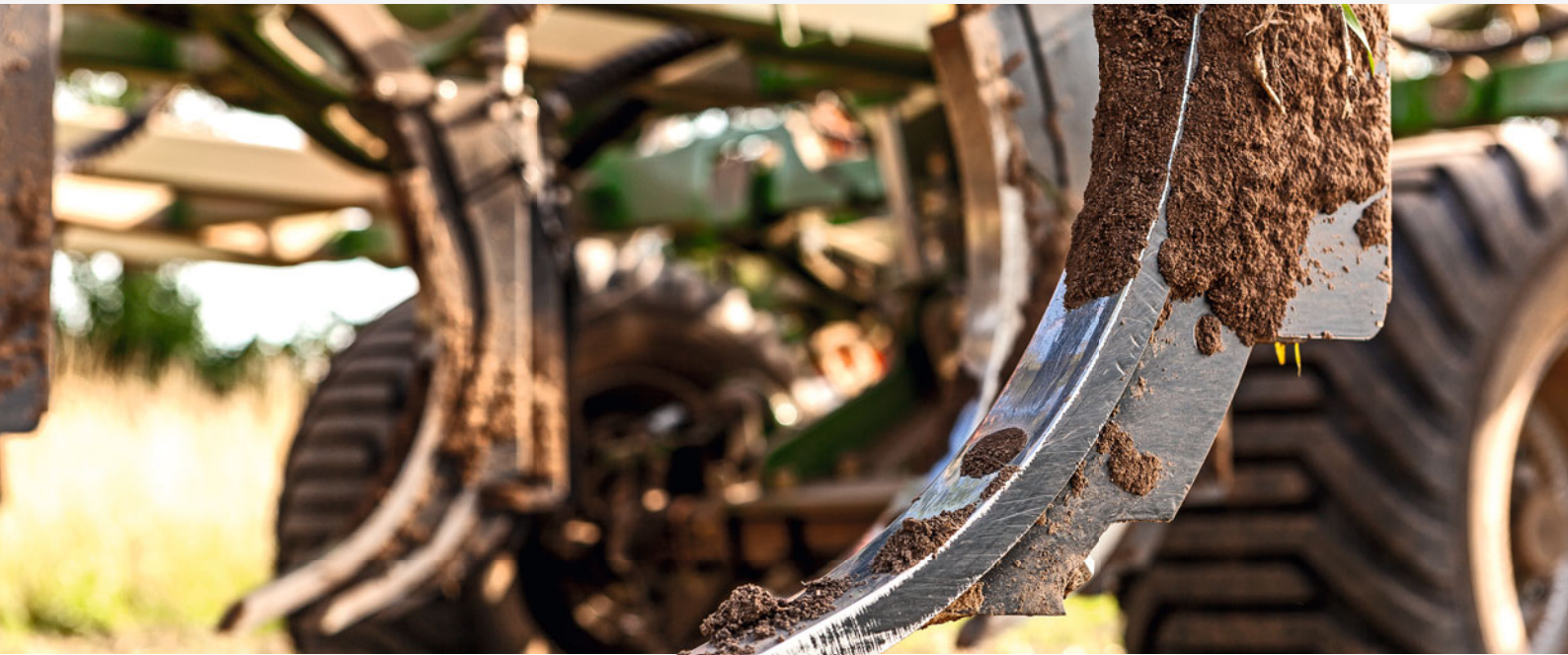
C-Mix coulter 40 mm with fertiliser supply tines for Cenius-2TX
