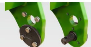
Cenius Special: C-Mix tines with shear bolt overload safety device and Angle profile roller
