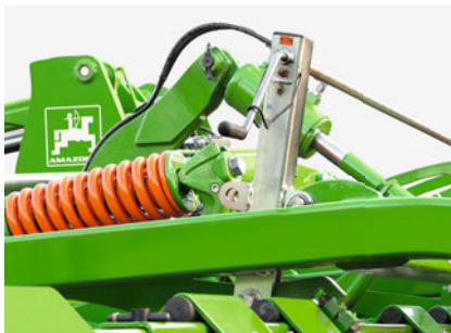
Spindles for the central adjustment of the levelling unit on the Cenius-2TX
