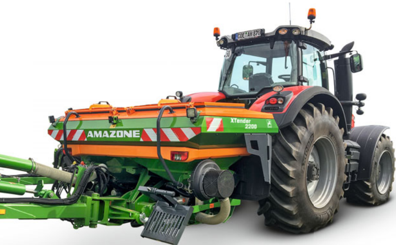
XTender 2200 mounted hopper in 2,200 l hopper capacity
