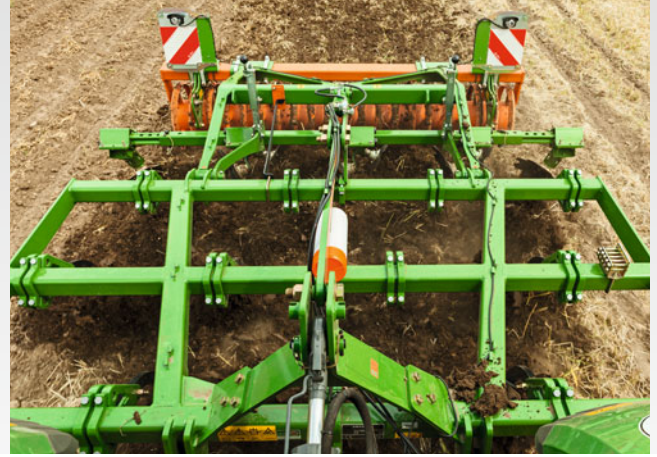
3-stagger frame mounting on the Cenius 3003 Special
