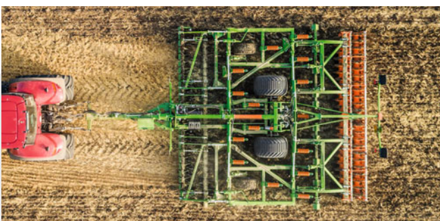
A tine runs behind each tyre to act as a track eradicator
