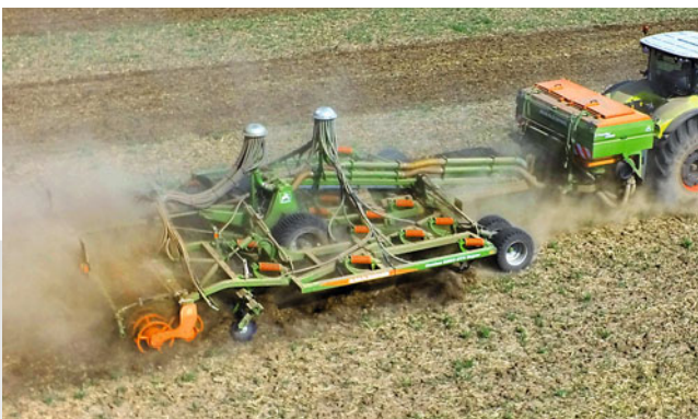
XTender 4200 with Cenius 6003-2TX and twin conveying systems for the application of fertiliser and seed
