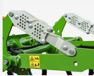
Mechanical working depth adjustment
