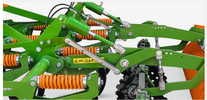
Automatic adjustment of the levelling unit
