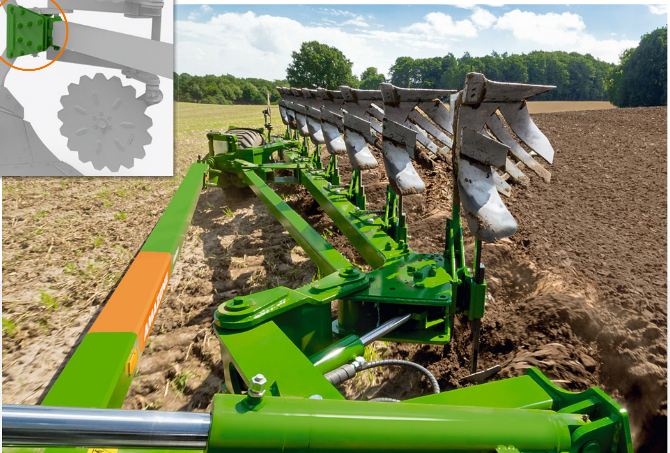
Shear bolt stone safety protection
