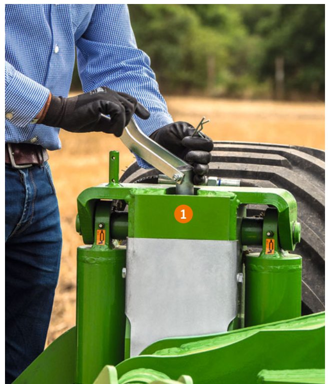
Working depth adjustment on the depth wheel
