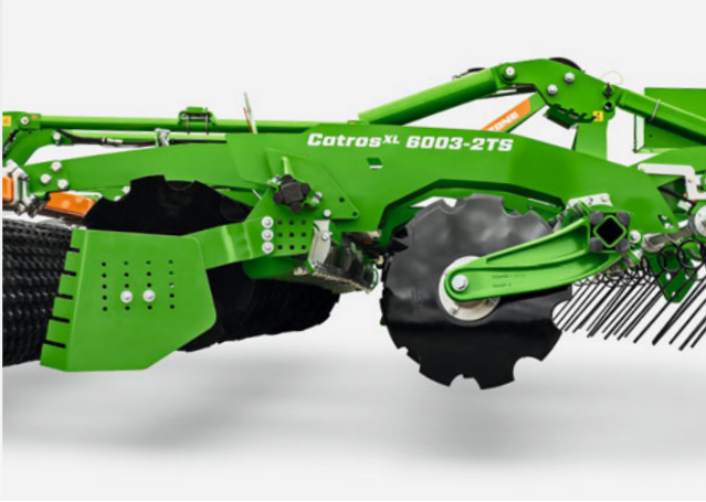
Catros XL 6003-2TS at its shallowest working depth – the discs are completely swivelled in towards the frame
