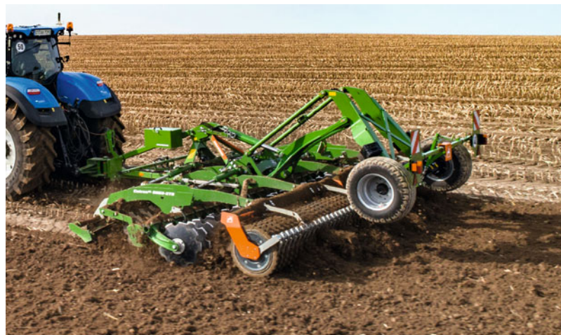
Catros XL 6003-2TS with up-front knife roller
