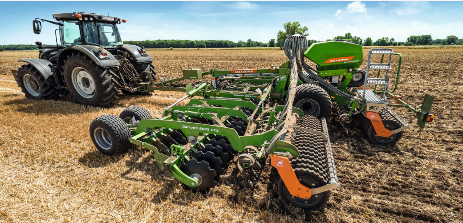
Catros XL 8003-2TX stubble cultivating with a top-mounted GreenDrill for catch crop sowing
