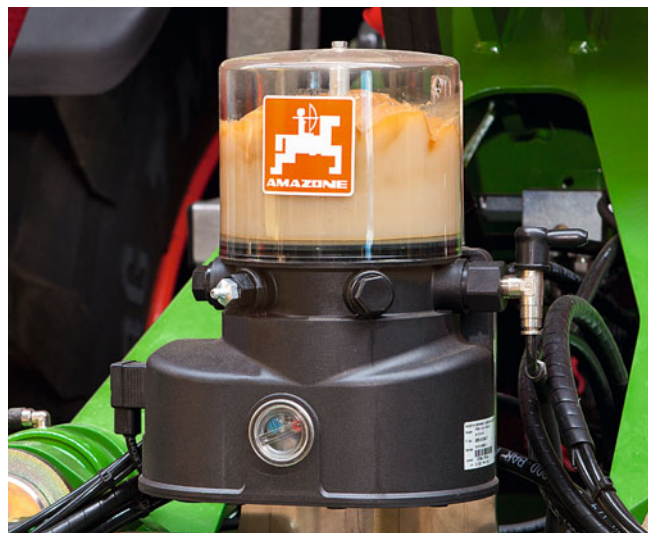
Pump with reservoir
